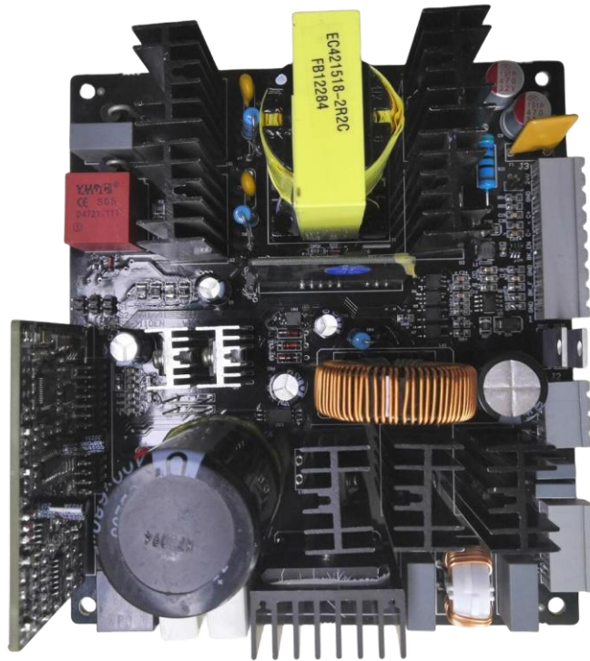
FIGURE 11.5 SJT-POBK-V1.3 brake & power supply board physical map
