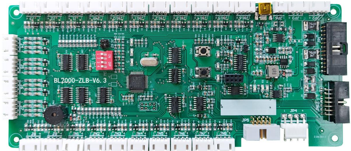
FIGURE 11.11 BL2000-ZLB-V6.x Car Instruction Board physical map
